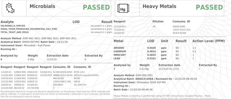
Heavy Metals screening is performed using ICP-MS (Inductively Coupled Plasma - Mass Spectrometer) which can screen to below single digit ppb concentrations for regulated heavy metals using method SOP-050 (R5). Sample preparation for Heavy Metals Analysis via SOP-050 (R5).
